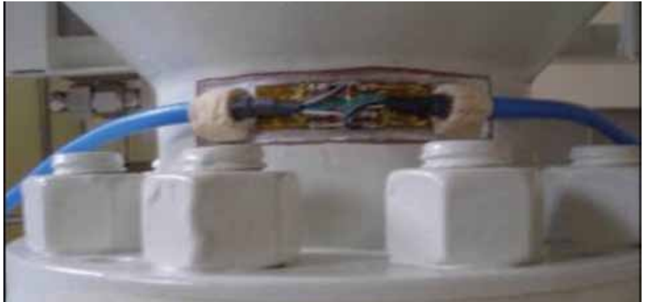
Installed Strain Gages.
