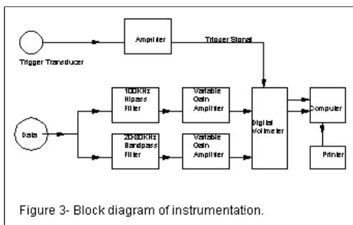
Figure 3- Block diagram of instrumentation.
