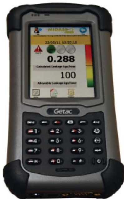
Figure 2: The hand-held ruggedized PDA, complete with proprietary leak estimation software.
