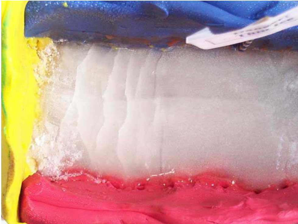
Figure 3. Photo of the ice at high deflection with cracks
